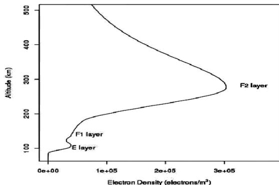
**Figure 1: The variation of electron density with altitude [6].**
